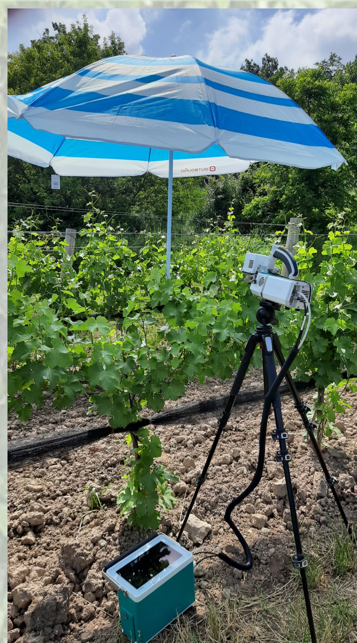
Fig. 1. The LI-6800 executing a temperature response program on a Vitis vinifera vine, in the Niagara vineyard.
