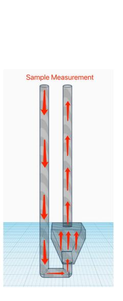
To satisfy the demand of a larger flow rate, the inner structure was designed as a double "U". The entrance/exit section of the pipelines are designed to fit a connector between the cuvette and the external tubing for a better seal. A small frame was added to the sides around the chamber to minimize contamination of the glue (used to adhere the glass to the cuvette) on the inside of the solution holding chamber.
